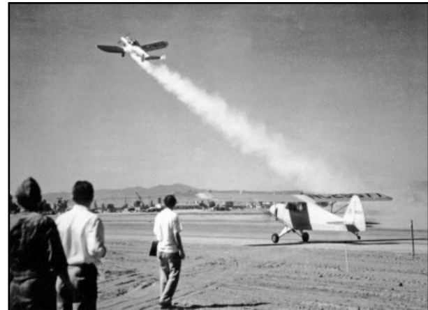
The Rocket Assisted Take Off of an Ercoupe at March AFB in August 1941.
